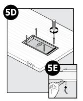
**5D** Use a screwdriver to evenly tighten screws throughout frame. It may be necessary to adjust screws to make sure pet door fit is correct.
