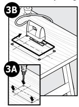
**3A** Drill %'' holes in inside corners of drawn template. These will be the pilot holes for the saw blade.
