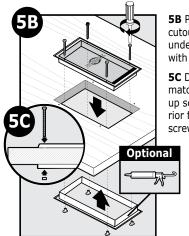
**5B** Place interior frame (frame with the flap) in cutout. Next place exterior frame into cutout from underside of the door. Hold frame pieces together with one hand.
