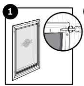
**To Replace** remove screws from the interior frame of pet door.
