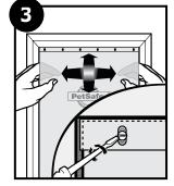
Replace new vinyl flap and position horizontally and vertically to fit into door frame. Replace existing bar and tighten screws in place.
